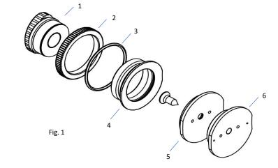
The 3206 XP AK+ Release valve is an auto-expulsion with push button suction easy to install component, and designed to be used with all suction suspension systems.
